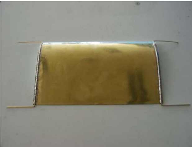
Wing section with metallic coating
