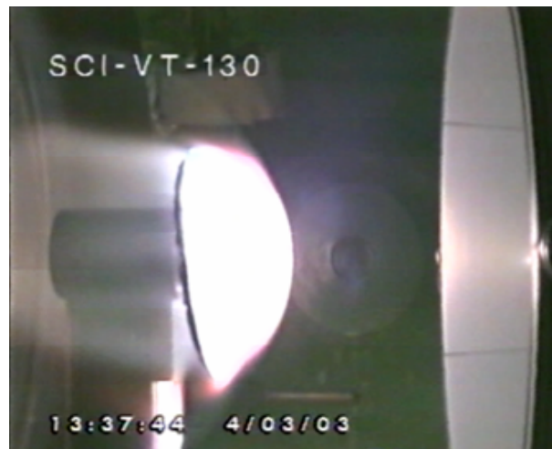
Figure 3. NASDA Hyflex test sample under test in flow condition. Total enthalpy: 11.9 MJ/Kg ; Stagnation pressure: 4.5bar
