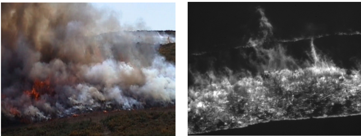
Figure 1.: (Left) Visible aspect of the 180 burn. (Right) The same scene in the 3,6 \mu\text{m} band. The fire front, propagating upward, is clearly seen.
