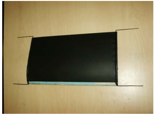
Wing section painted with measured emissivity paint
