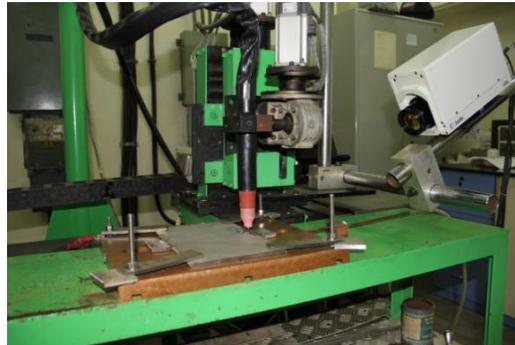
**Fig. 1.** Title TIG welding machine setup with IR camera
