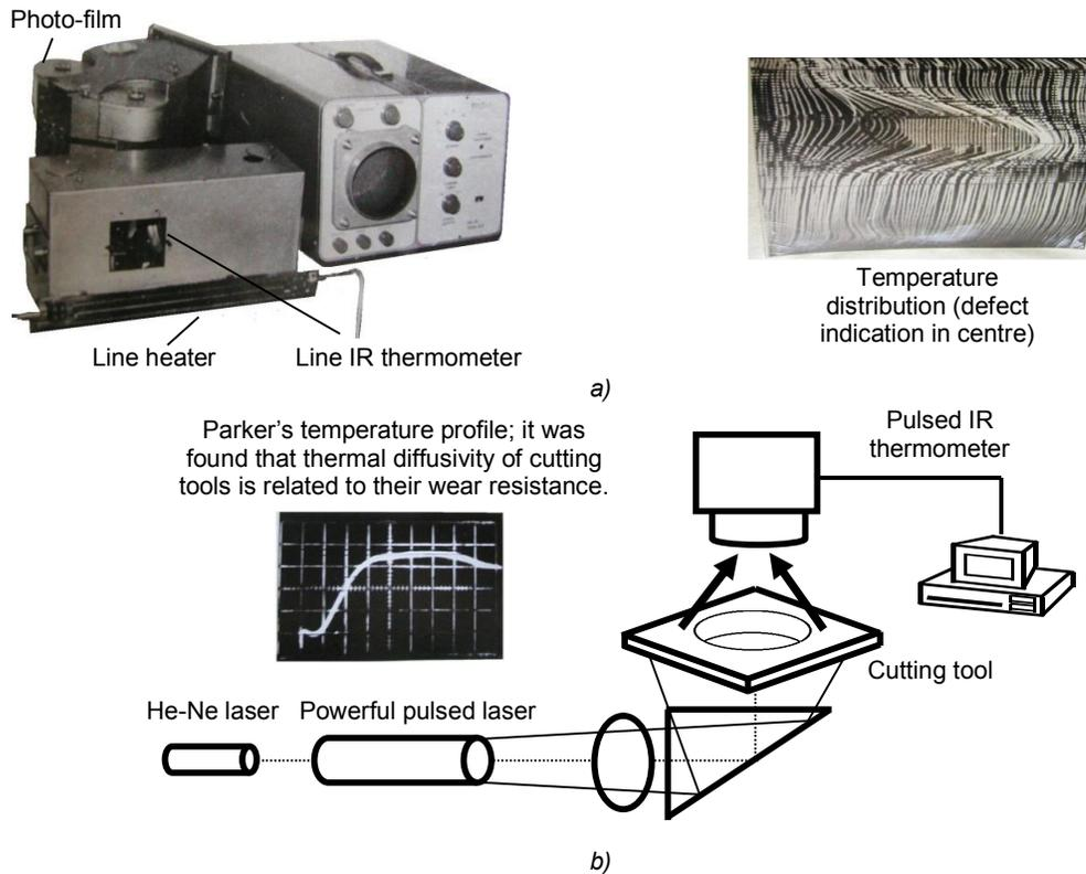
**Fig. 1.** Specialized TNDT equipment, Tomsk Polytechnic University:
