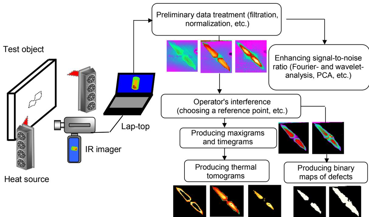
**Fig. 4.** Thermal tomographic unit for inspecting composites
