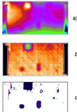
Data processing examples in TNDT of CFRP composite: a-source image, b- Fourier phasegram, c-thermal tomogram of the 1.1-1.3 mm layer
