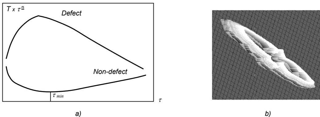
**Fig. 2.**  $T(\tau) \times \tau^n$  concept: a) evolution in time, b) reference-free thermal tomogram of impact damage in CFRP
