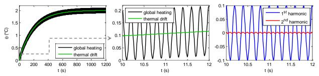
Fig. 1: Time-evolution of a simulated heating signal of a sample under cyclic loading of fixed amplitude and frequency.
