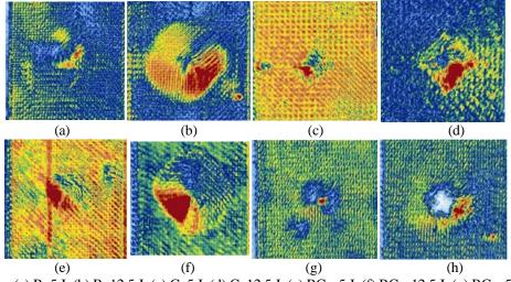
Figure 1: UT results: (a) B: 5 J, (b) B: 12.5 J, (c) C: 5 J, (d) C: 12.5 J, (e) BCs: 5 J, (f) BCs: 12.5 J, (g) BCa: 5 J, (h) BCa: 12.5 J.
