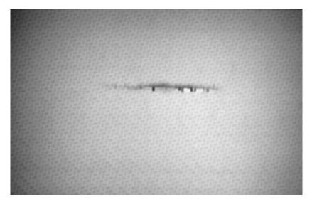
Fig. 2 Thermogram of single plate after shoot lead projectile (transmission approach).
