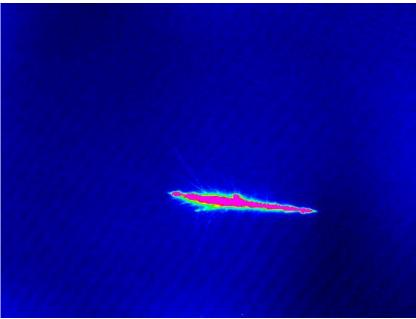
Fig. 1 Thermogram of single plate after shoot lead projectile.
