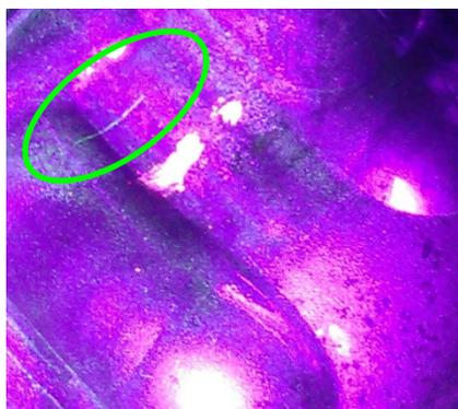
**Fig. 1:** Steel part under magnetic particle inspection. The crack is indicated with a green marker.
