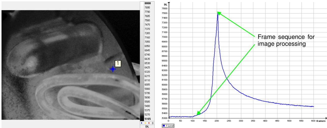
**Fig. 4:** Example of time evolution for a given pixel in the induction area next to the coil.
