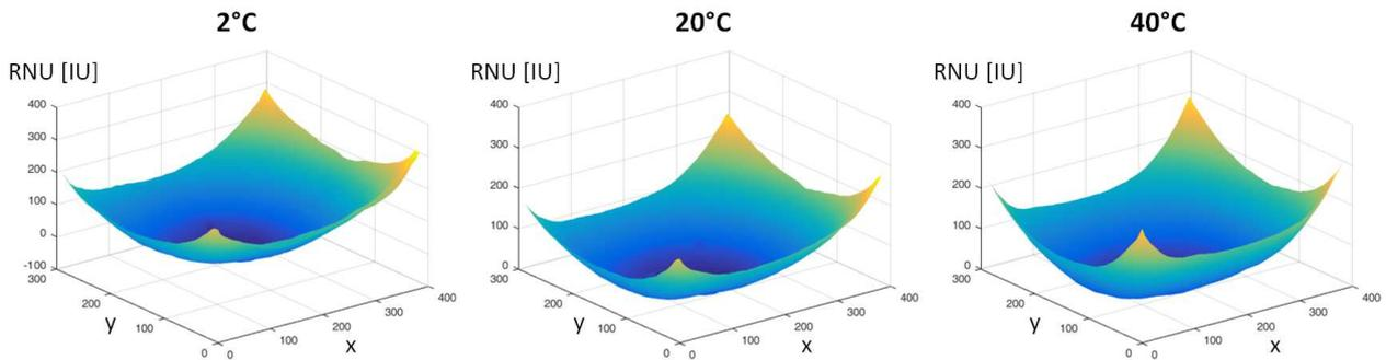
Fig. 2. 3D visualisation of RNU characteristics for different temperature conditions of working camera
