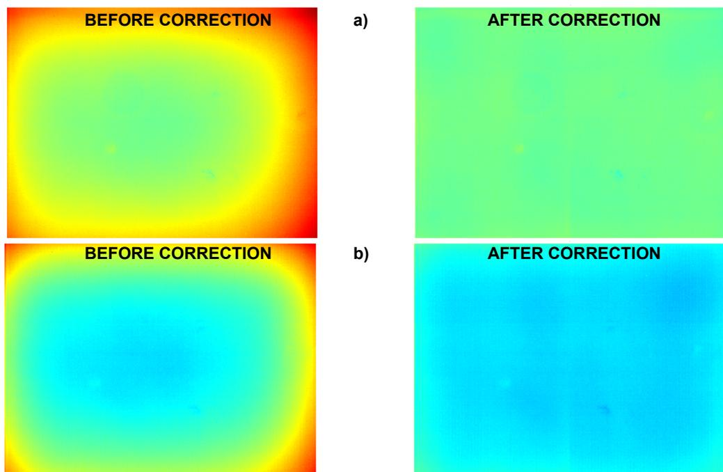
**Fig. 4.** False color images of black body (set to 40°C) before and after developed RNU correction for two different temperatures of camera working environment. a)  $T_{ambient}=20^{\circ}C$  b)  $T_{ambient}=40^{\circ}C$
