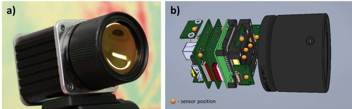
**Fig. 1.** The designed infrared camera (a) and its perspective view of interior with marked sensors positions (b)
