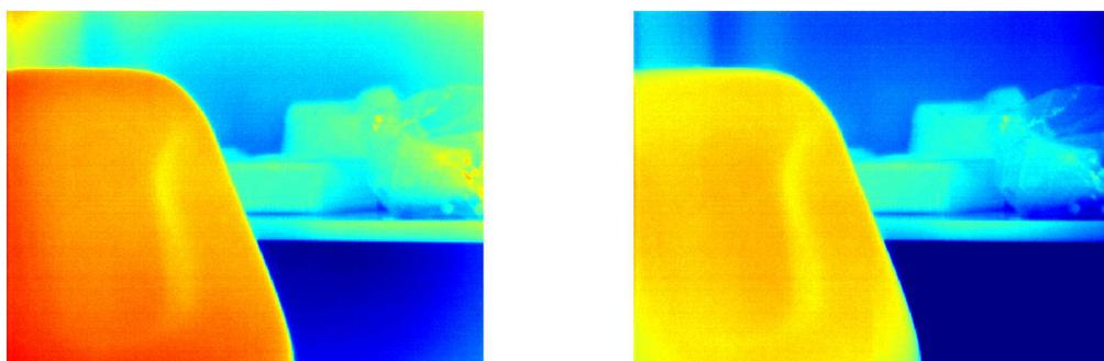
**Fig. 5.** False color images of office interior before and after developed RNU correction
