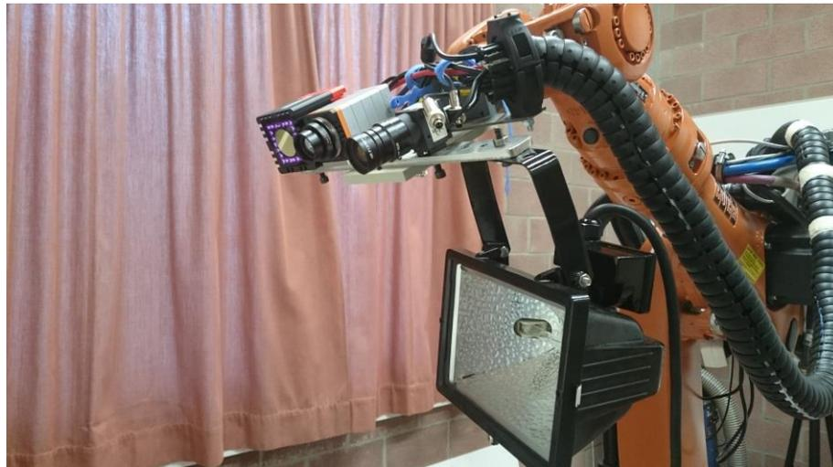
**Fig. 2.** Three-dimensional thermal imaging system existing of a MESA SR4000 time-of-flight camera (left), a XENICS Gobi 640 thermal camera (middle), a CMOS uEye UI124xSE RGB camera and a 500 Watt halogen light.
