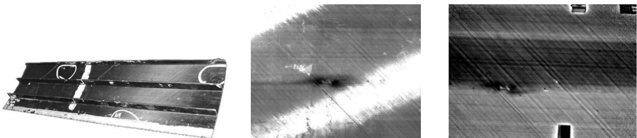
**Fig. 4.** Curved CFRP landing flap. Photograph (left), Halogen lamp (center) and VCSEL (right) excited lock-in thermography results.
