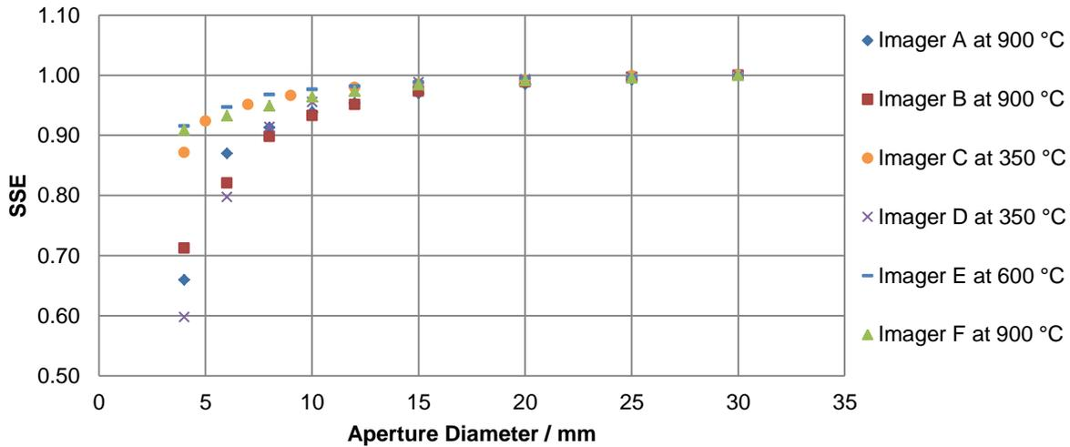
Fig. 5 High temperature SSE results.
