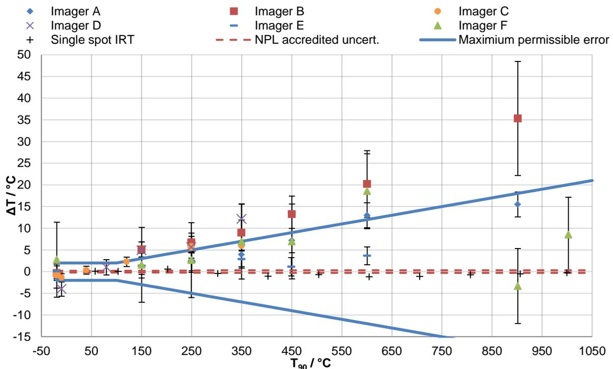
**Fig. 2** Calibration results for the thermal imagers at a distance of 1.0 m. The solid line shows most manufacturers' stated uncertainties and the dashed line shows NPL's accredited uncertainty ( $\leq 0.3$  °C below 1000 °C). For comparison the calibration results for a single spot infrared radiation thermometer are also shown.
