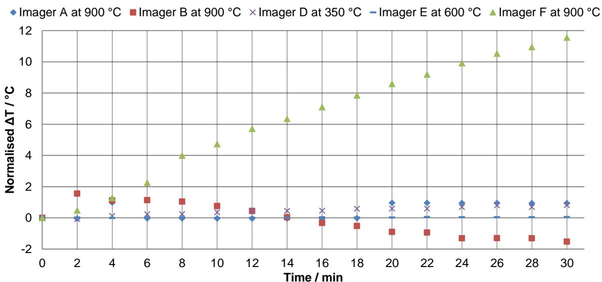
**Fig. 7** Measurement of thermal imager’s drift over a 30 minute period after ‘switch on’.
