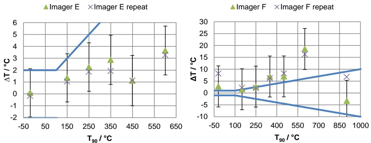
**Fig. 3** Repeatability of two thermal imagers; (left) imager E showing good repeatability, (right) imager F showing poor repeatability at the bottom and top of its range. For the Y-axis  $\Delta T = T_{90} - T_{\text{imager}}$ . The solid line indicates the manufacturers' stated uncertainty and errors bars represent the NPL calibration uncertainty.
