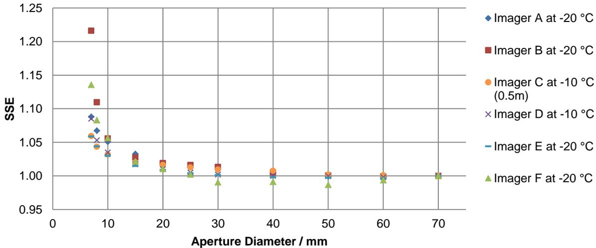
Fig. 6 Low temperature SSE results.
