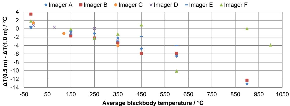
**Fig. 4** The effect of distance on thermal imager temperature readings.
