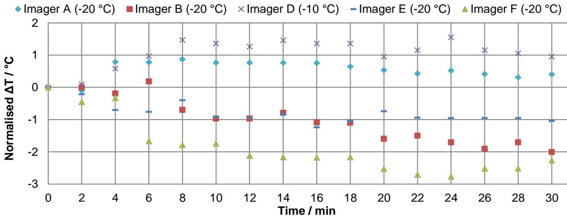
Fig. 8 Measurement of thermal imager’s drift over a 30 minute period after ‘switch on’, imager’s minimum measurable temperature.
