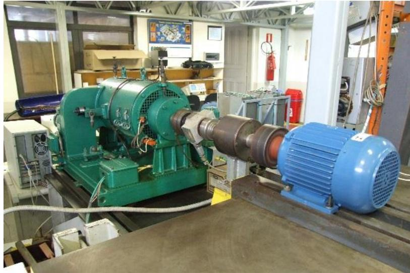
Figure 6 – Motor test bench
