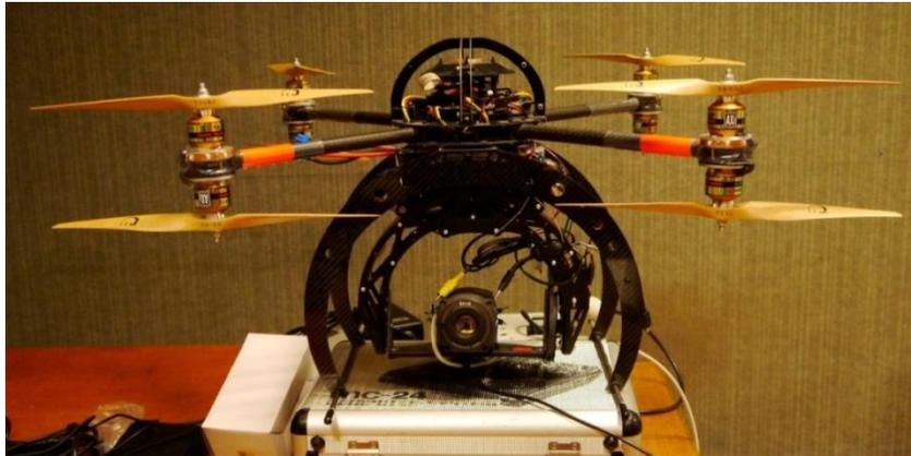
**Fig 1.** UAV (Push-Pull Octocopter DS8X-N3) equipped with an IR camera (Flir A320G)
