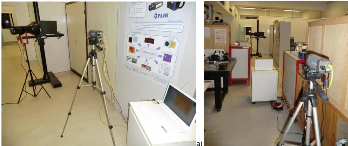
**Fig 3.** Preliminary experimental setup (front face impulse IR testing). From left to right: camera located at (a) 2 m and (b) 8 m distance from the sample.
