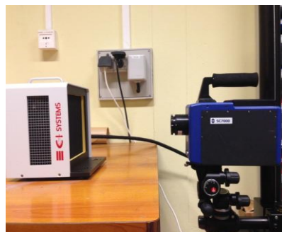
Fig. 7. IR camera facing the black body
