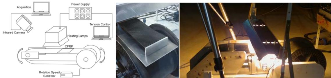
**Fig. 6.** From the left to the right, a diagram and pictures of the experimental setup to test the implementation of the heating process as well as the thermography system.
