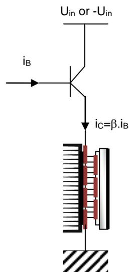
**Fig. 4.** Usual amplifying circuit principle
