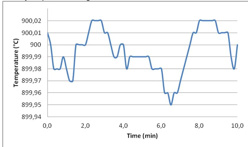
**Fig. 9:** example of stability curve of the temperature over 10 minutes at  $900^{\circ}\text{C}$
