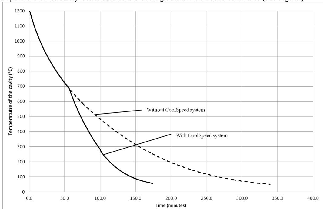
**Figure 11: Cooling curve of a cavity blackbody from 1200°C without and with CoolSpeed system**
