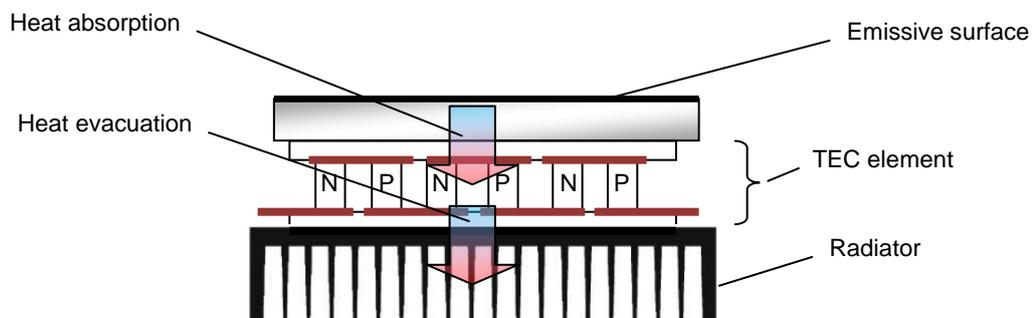
*Fig. 1. Low temperature emissive head principle*
