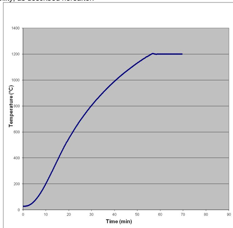
**Fig. 8:** rising time from ambient temperature to 1200°C
