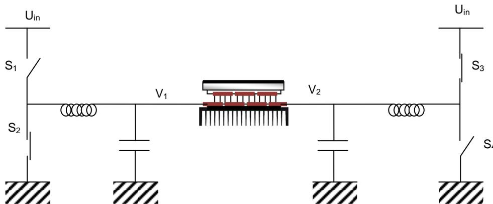
Fig. 5. High efficiency amplifying circuit principle
