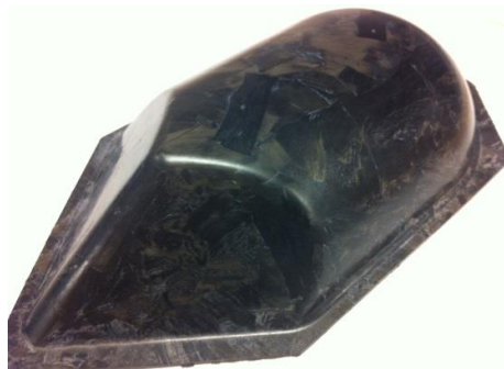
Figure 1 - Complex shaped part moulded with random-oriented strands (ROS)
