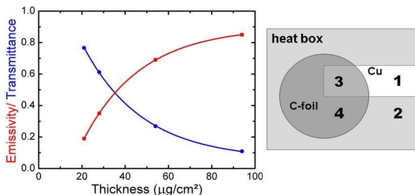
**Fig. 1.** Measured emissivity and transmittance (left) values for foils of different thicknesses and radiance measurement setup (right).
