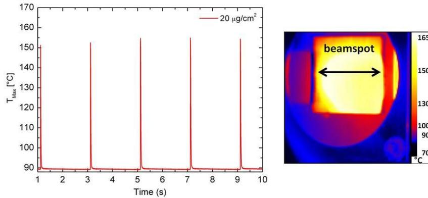
**Fig. 2.** Time evolution (left) and spatial gradient (right) of temperature in the beam spot during irradiation of a 30  $\mu\text{g}/\text{cm}^2$  carbon foil with a 1.1 GeV U ions.
