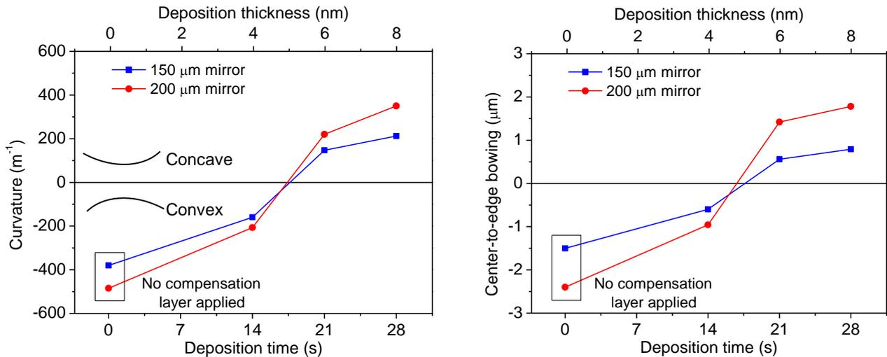
**Fig. 6.** (a) Curvature, and (b) center-to-edge bowing of released filter as a function of SiN<sub>x</sub> compensating layer thickness. Curvature is defined as reciprocal of radius of curvature.
