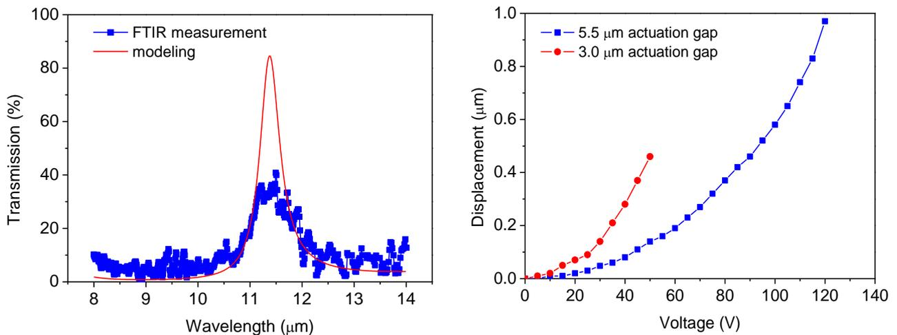
**Fig. 7.** (a) FTIR transmission measurement of fabricated  $150\text{ }\mu\text{m}$  diameter filter with  $550\text{ nm}$  center-to-edge bowing, and (b) displacement of  $200\text{ }\mu\text{m}$  long doubly-clamped beam actuators
