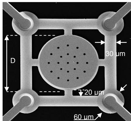
**Fig. 5.** SEM image of a fabricated LWIR filter and its structure dimensions
