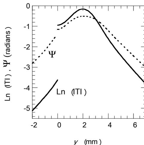
**Fig. 2** Surface temperature profile (amplitude and phase) along the  $y$  direction for an infinite vertical crack with  $R = 10^{-3} \text{ m}^2 \text{ K/W}$ . Calculations are performed for AISI-304 at  $f = 0.8 \text{ Hz}$ , using a laser beam of radius  $0.5 \text{ mm}$ ,  $d = 2 \text{ mm}$ .
