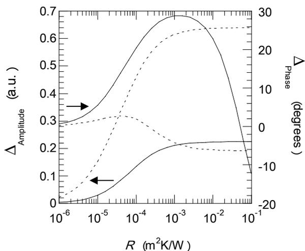
**Fig. 3.** Amplitude and phase contrast as a function of thermal resistance, for an AISI-304 sample excited by a modulated ( $f = 0.8 \text{ Hz}$ ) laser of radius  $0.5 \text{ mm}$ . Continuous line stands for  $d = 1 \text{ mm}$  and dotted line for  $d = 0.3 \text{ mm}$ .
