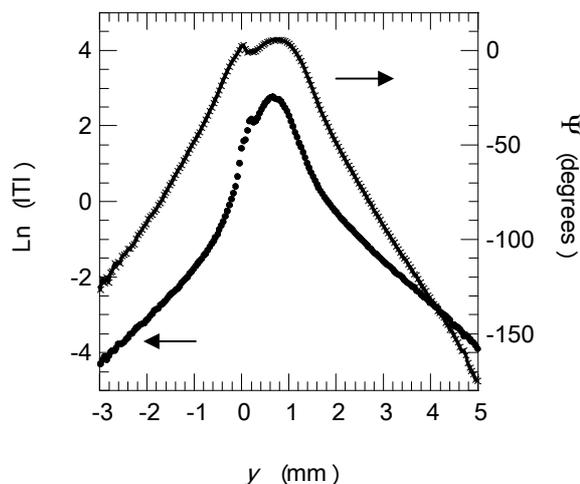
**Fig. 4.** Amplitude and phase temperature profiles along the  $y$  direction for an AISI-304 sample with an infinite crack  $25 \mu\text{m}$  thick ( $R = 10^{-3} \text{ m}^2 \text{ K/W}$ ) measured at  $0.8 \text{ Hz}$ .
