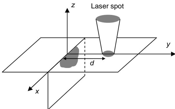
**Fig. 1.** Scheme of the vertical crack on a semi-infinite sample.
