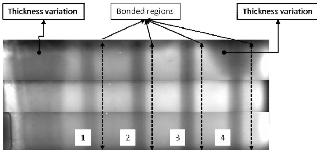
Figure 11. Thermal image of aircraft component obtained after scanning
