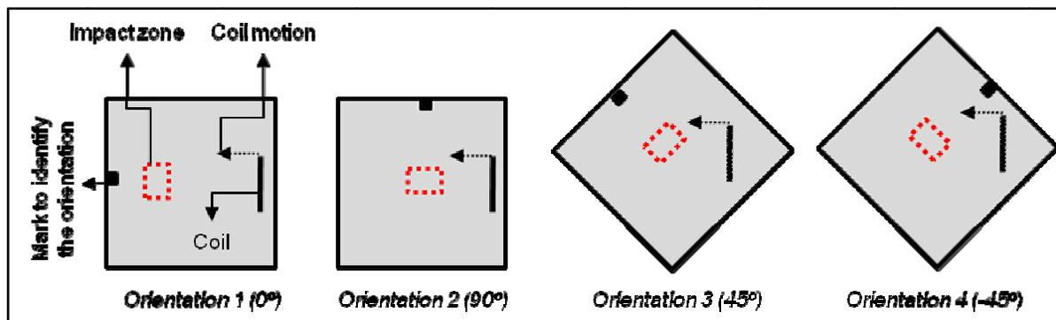
Figure 3. Different specimen orientation for performing SIT
