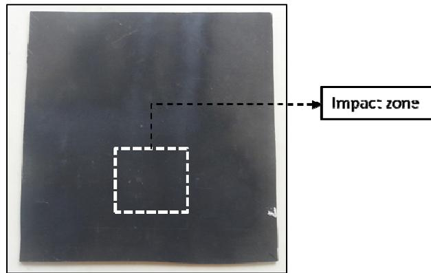
Figure 2. Real image of CFRP panel. The impact zone is shown in the image
