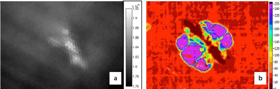
Figure 9 a: Final image obtained by rotating and merging all the four images; b: Ultrasonic scanning result of impact damaged zone
