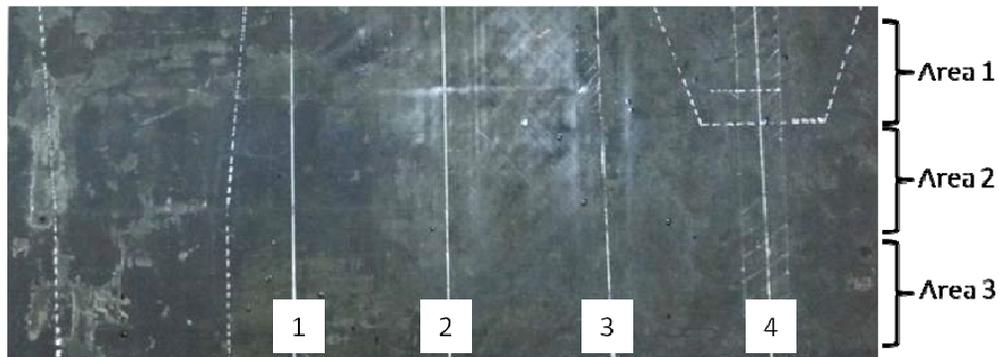
Figure 10. Real image of scanned aircraft component. Locations of stiffeners are marked as 1, 2, 3 and 4; Scanned regions are marked as Area 1, Area 2 and Area 3.
