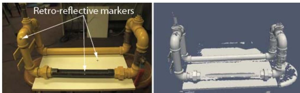
Fig. 3 Pipe structure with retro-reflective markers (left). Shaded 3D model measured by the handheld 3D scanner (right)
