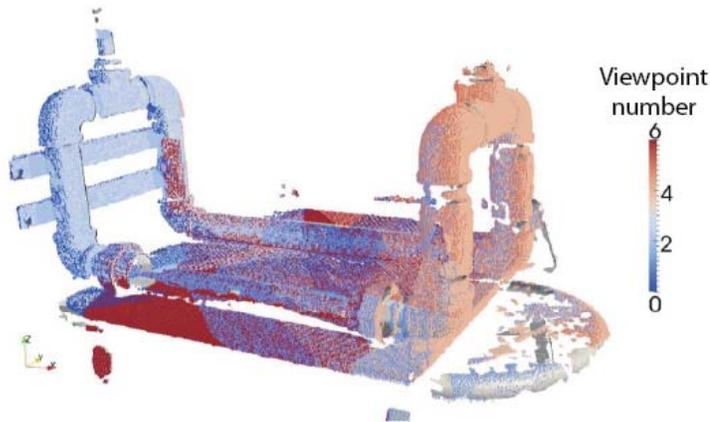
*Fig. 11 3D Pipe model with colors indicating from which point of view the thermal measurement was captured*
