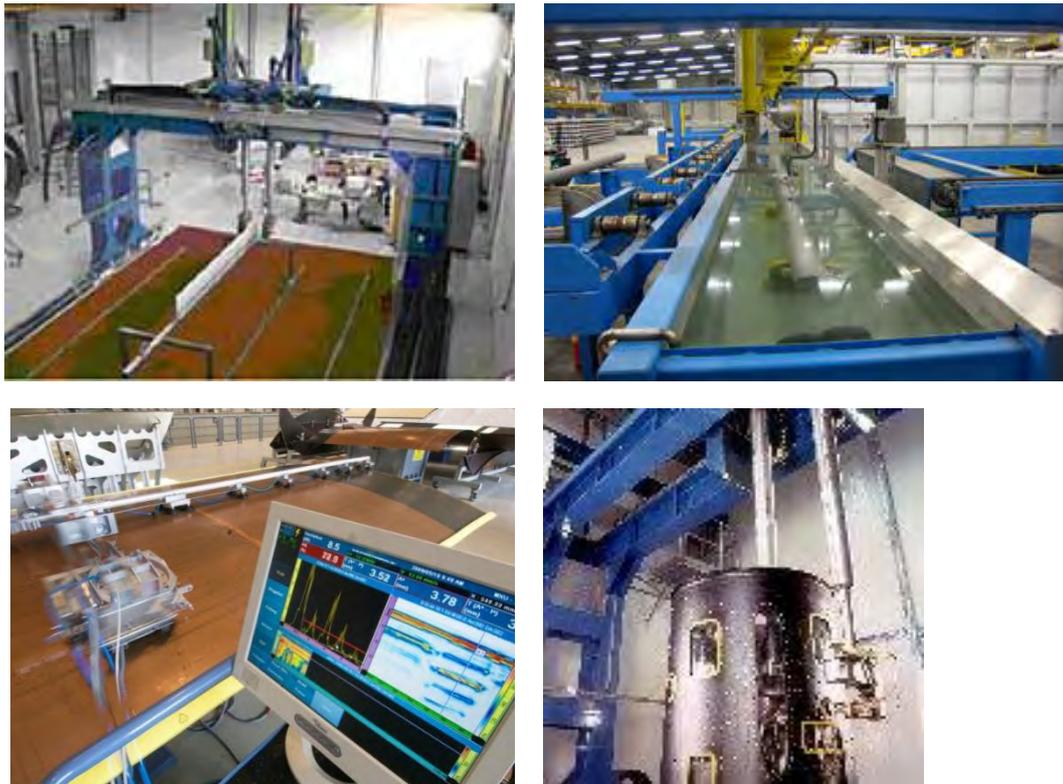
Fig 5 Examples for water coupled ultrasonic inspection (sources: National Composites Network, Premium Aerotec, IntelligeNDT, HPI)
