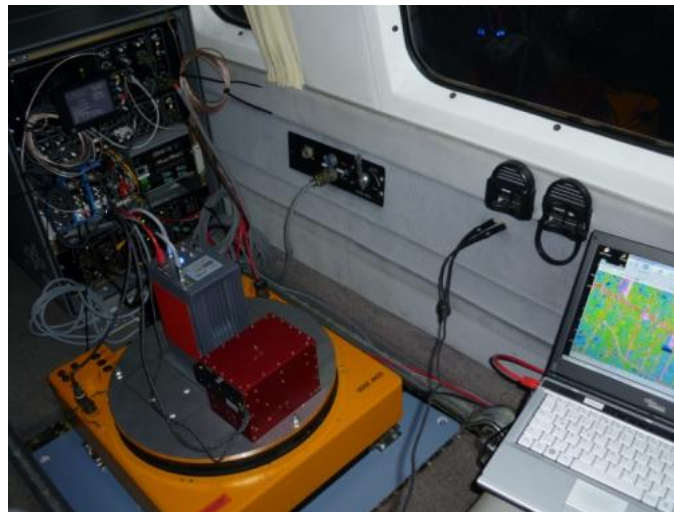
Fig. 8. Setup inside aircraft during data acquisition. ImageIR 8300 mounted lens down on stabilization platform, IMU mounted next to camera, auxiliary hardware inside rack, laptop showing actual thermal images
