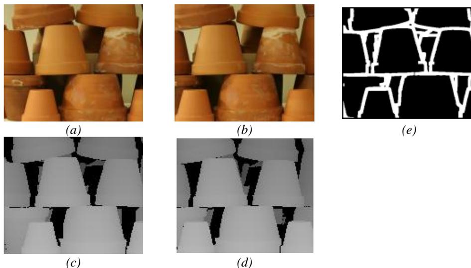
**Fig. 1.** Stereo Vision Systems where (a) camera image right (b) Left camera image (c) disparity map right (d) disparity map left (e) merged boundaries of occlusion.
