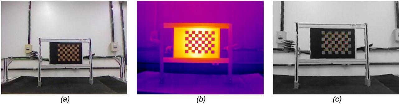
Fig. 5. Calibration Rig: 320x240 resolution visible (a) 640x480 thermal image (b) reprojection of calibrated points (c)
