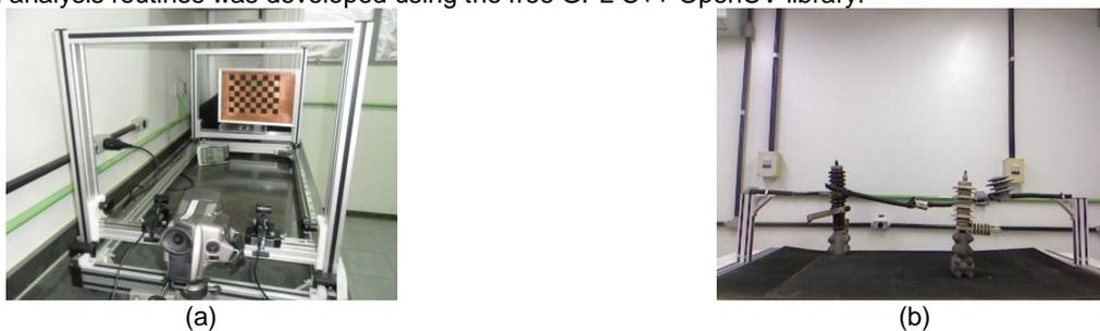
**Fig. 4.** Stereo vision system prototipe (a) and test bench (b)
