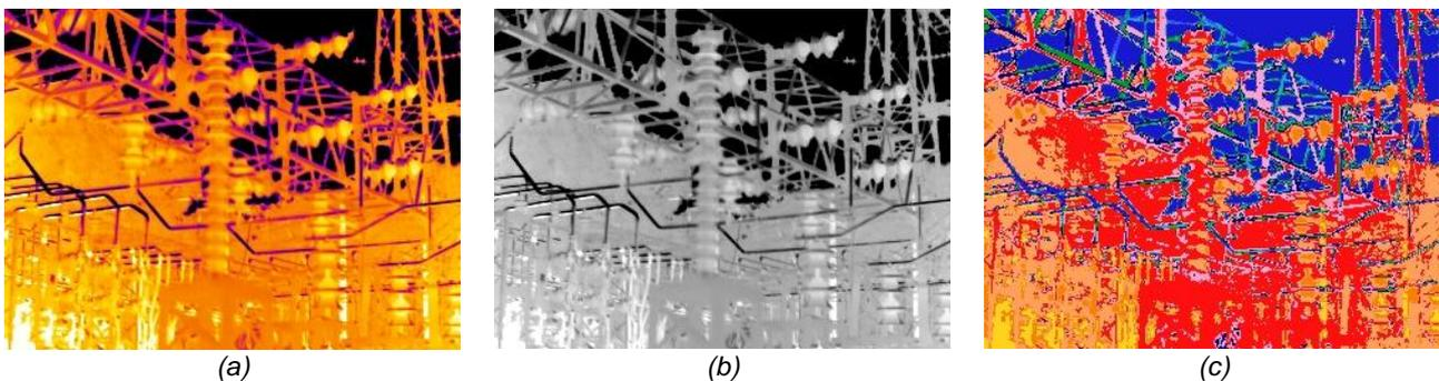
Fig. 3. Thermal imaging of surge arresters in different pallets (courtesy of CEMIG S/A)
