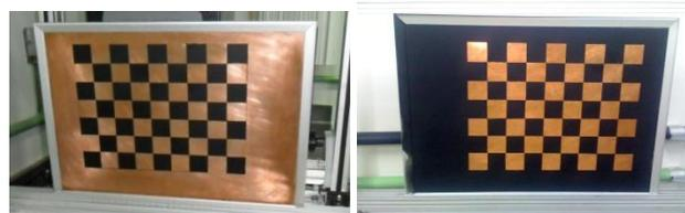
Fig. 1. Calibration Rigs
