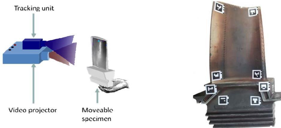
**Fig. 7. Left:** Schematic view of Real-View setup for dynamic case.
