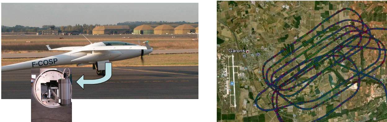
Fig. 6. Left : camera A325 installed in the right pod (shown opened in the small view) of the STEMME motorglider. Right : View of the five flight lines over the Garons area (mean coordinates: 43°46'N, 42°7'E).
