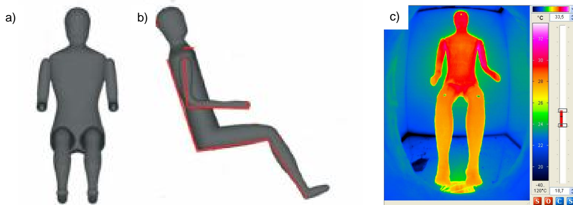
Fig. 3. Thermal passenger dummies a) front view, b) side view and c) inside a test environment for approval of the technical specifications
