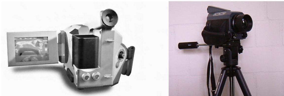
Fig. 2. Portable thermographic test equipment
