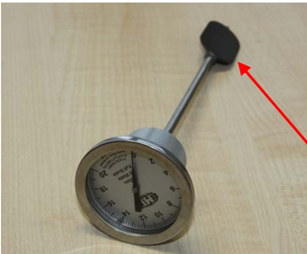
Fig. 6: power meter P 20 from Macken Instruments, the arrow points to the sensitive zone
