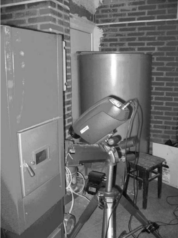
**Fig. 6.** Test boiler for shredded sorghum equipped with infrared monitoring system
