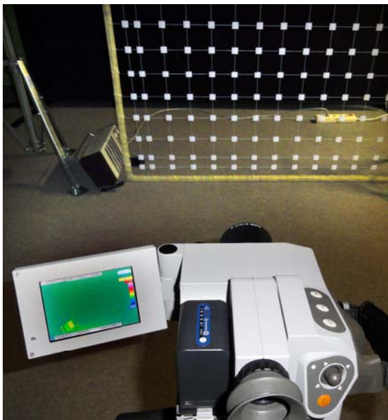
Fig. 3. The photography of the equipment from measuring of temperature fields in 3D airflow with measuring targets by an infrared camera
