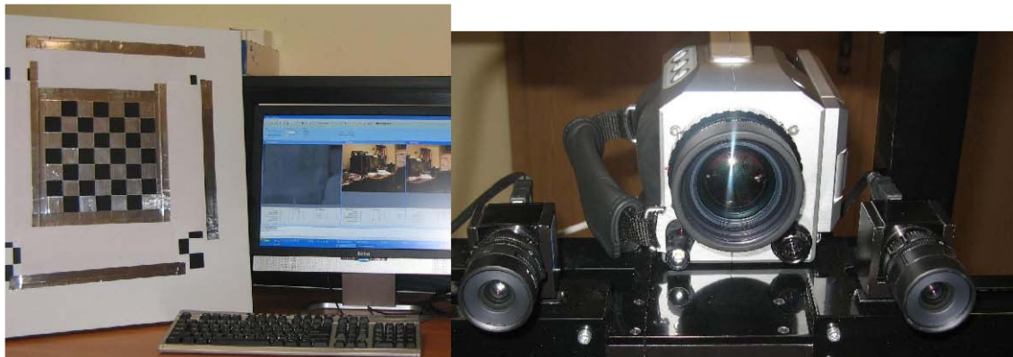
Fig. 1 Calibration Board and the set of the three cameras: thermal and visual ones.
