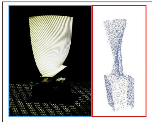
*Fig. 1: Blade with fringes and Pointcloud of the blade*
