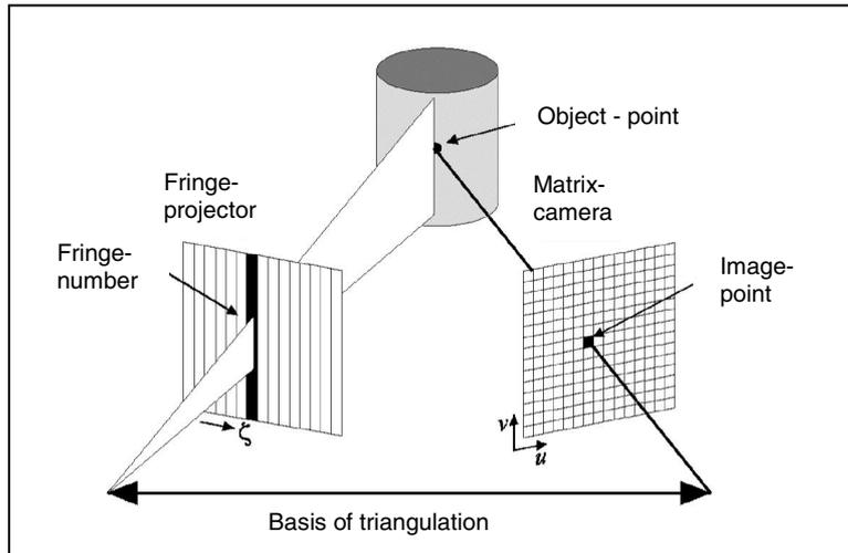
**Fig 2:** Principle of fringe projection
