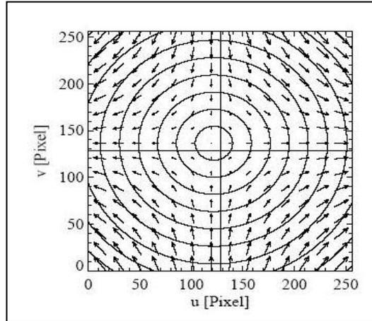
**Fig 4:** Correction field for the distortion of an optical camera
