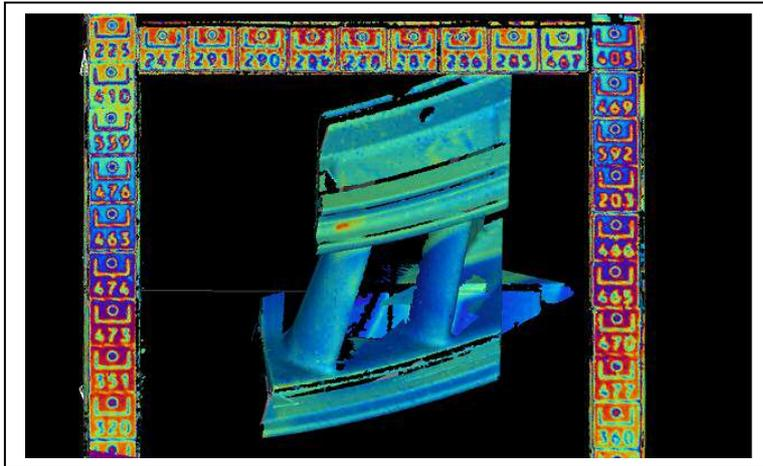
**Fig 9:** Image of the 3d point cloud textured with the thermographic data image 7, using pixel rays. This technique is similar to the ray tracing methods
