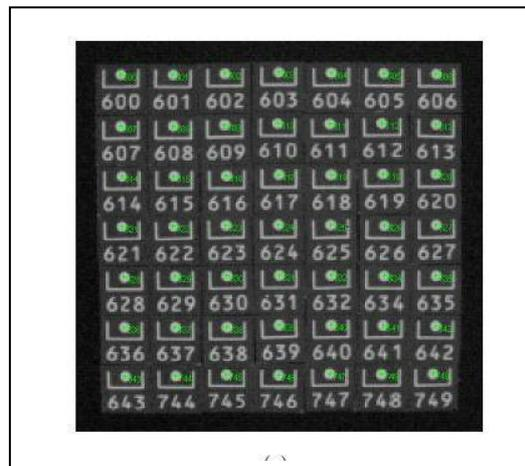
**Fig. 5:** A calibration plate, which can be used in the optical and infrared regime
