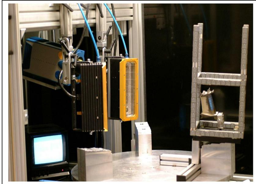
**Fig 6:** The thermographic equipment, the specimen and the cage. The infrared camera also records the optical marks. Since this camera is photogrammetric calibrated it is possible to calculate the position of the camera relative to the cage.
