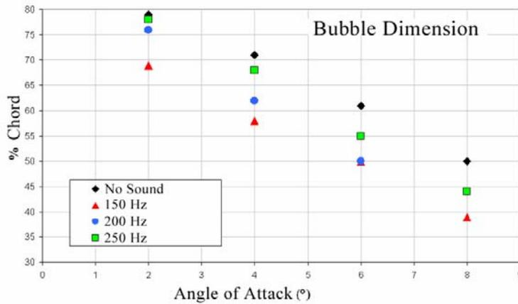
Fig. 10 Modification of the Laminar Bubble Dimension by varying the Woofer frequency (Re=60k)
