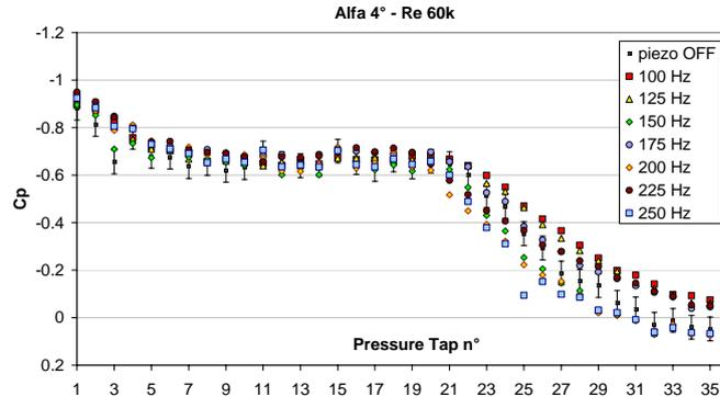
Fig. 12 Pressure distribution analysis for  $\alpha 4^\circ$  and Reynolds 60k
