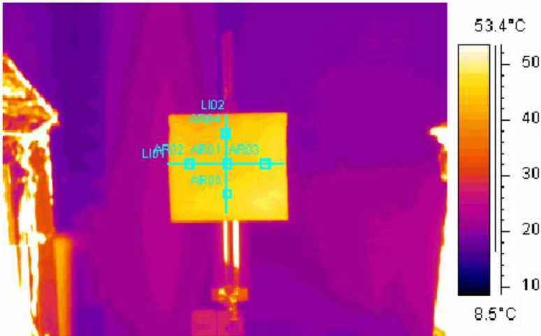
*Fig. 3. Infrared image of the first sample at the end of the thermal excitation.*
