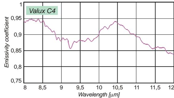
Fig. 3. Emissivity coefficient of an example dental material
