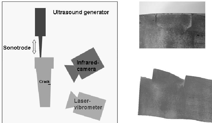
**Fig. 1.** Left: Ultrasound excited thermography on turbine blades. Right: Photograph of an area with two cracks (top) and result of an experimental vibration analysis (bottom)
