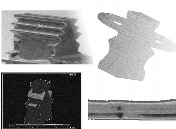
**Fig. 2.** Upper left: Photograph of a turbine blade root with a 1 mm long crack in the indicated area. Upper right: Modelling of the blade root and the induction coil. Lower left: Calculated temperature distribution. Lower right: Enlarged thermographic image of the tested area. The crack becomes visible.
