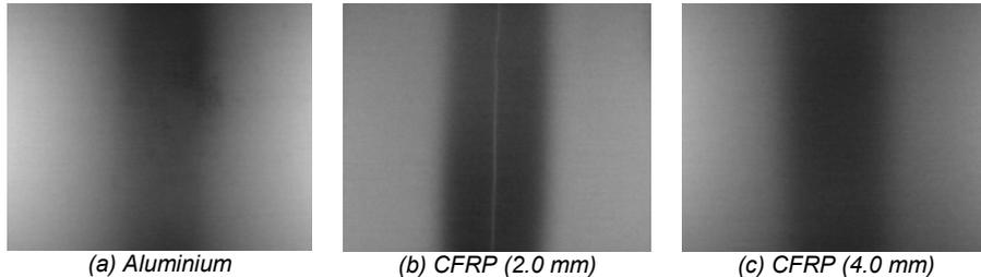
**Fig. 8.** Thermal images obtained from the miniature Omega camera system.
