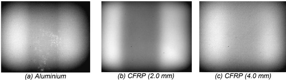
**Fig. 6.** Thermal images obtained using the ThermoScope system
