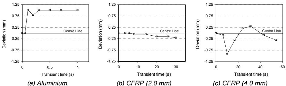
**Fig. 7.** Accuracy analysis of the centre line detection algorithm
