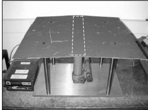
**Fig. 2.** *The experimental set-up for testing various skin-strut combinations.*
