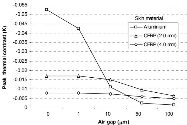
**Fig. 4.** Thermal modeling results of peak contrast as a function of air gap for both the aluminium and CFRP models.
