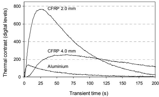
**Fig. 5.** Contrast-time plots for the aluminium and CFRP skins
