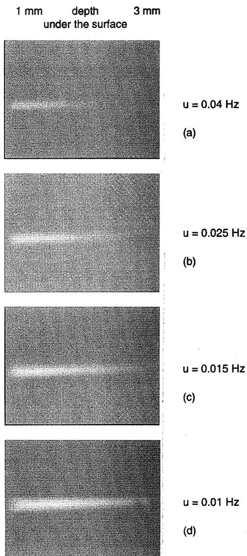
*figure 1* Phase images obtained with the PPT approach at various frequencies over a plastic specimen with an inclined slot of 6.4 mm width and of variable depth as shown.
