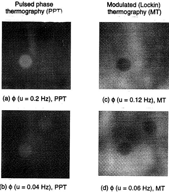
*figure 2* Phase images obtained with both PPT (left) and MT (right) approach at various frequencies over a graphite epoxy plate with two-embedded Teflon® implants of 10 mm in diameter located at about 2 and 3 mm under the front surface (different image sizes and operating distances).
