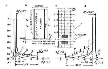
a — changes of the surface temperature on the cold side, b — model of the joint, c — network diagram, d — changes of the surface temperature on the warm side; for infiltration: 0 — experiment, 1, 2 — calculation for  $\alpha_{pn}=0.058~\rm W.m^{-1}.K^{-1}$  and  $\alpha_p=0.189$ , respectively; for exfiltration: 3 — experiment, 4, 5 — calculation for  $\alpha_{pn}=0.05$  and  $\alpha_p=0.151$ , respectively
