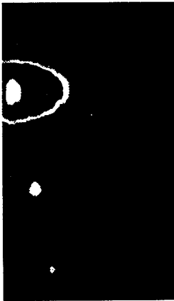
a - cross-sectional timegram for two defects at the depth 1.8 and 3.6 mm
